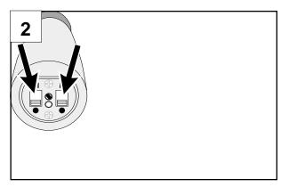
Turn the transmitter Power "P" on and Microphone "M" on by sliding the switches toward the dots.
